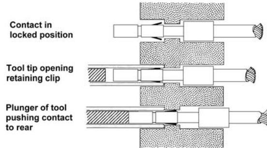
3. Insert Lock - the contact has a ridge (shoulder) machined around the contact which snaps into place in the spring clips (tines) located inside each cavity of the insert. The contacts are usually inserted from the rear of the connector and removed either from the front or rear of the connector.
